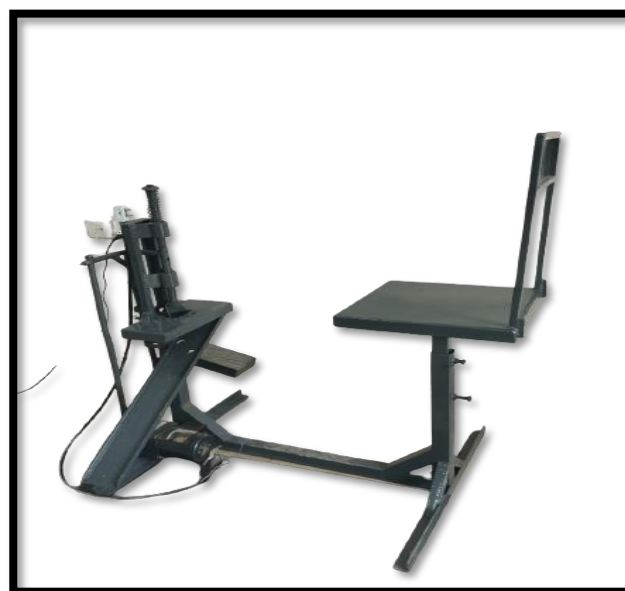
Figure 3: Motor and manual operated sugarcane bud chipper machine
