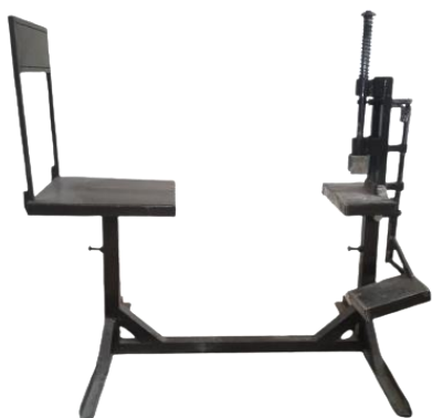
Figure 2: Manual Operated Sugarcane Bud Chip Cutting Machine
