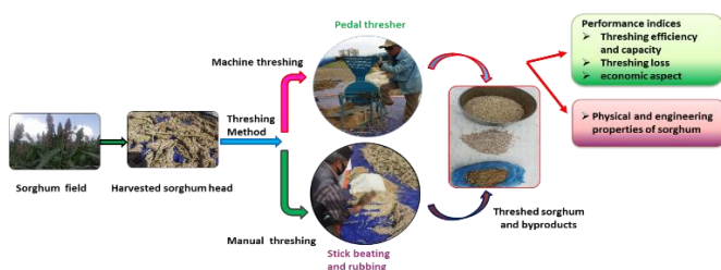
Figure 3: Schematic diagram of experimental set up for sorghum threshing in this study
