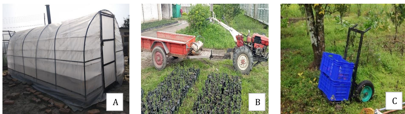
Figure 7: NAERC Developed Solar Tunnel Dryer (A), Power Tiller with Trailer Attachment (B) and Portable Wheel Trolley (C)
