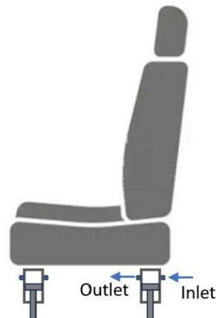
Figure 5: The piston systems are mounted underneath the seat of the vehicle
