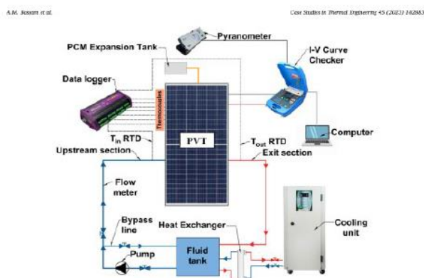
Figure 1: schematic diagram of a Photovoltaic/Thermal (PVT) experimental
